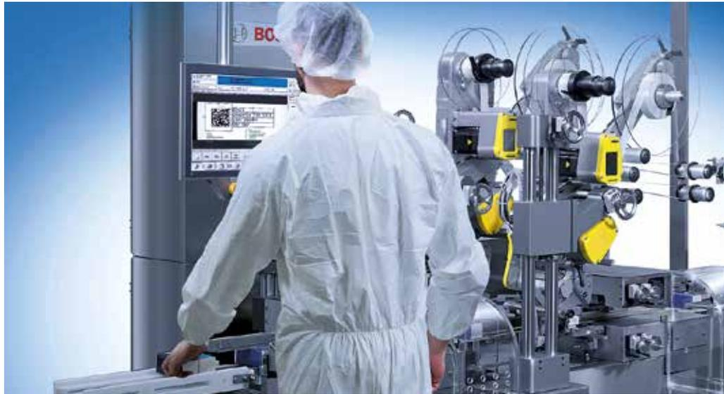
Modern packaging machinery equips pharmaceutical packages with Data Matrix Codes and tamper-evident safety seals.
